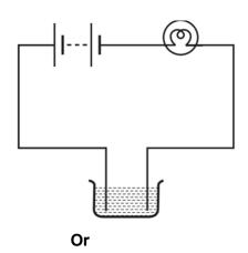
In case of a fire, before the firemen use the water hoses, they shut off the main electrical supply for the area. Explain why they do this.
