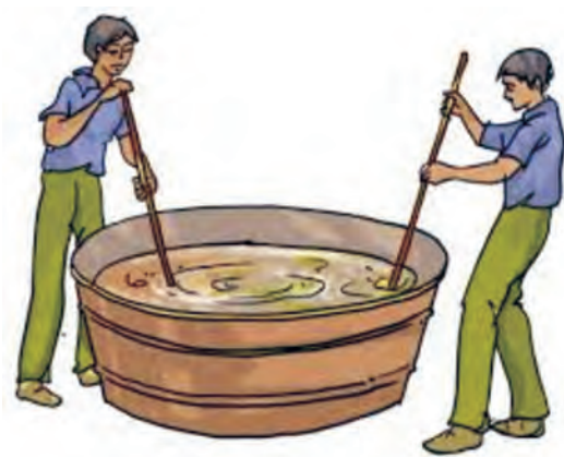
Fig 3.8 (a) Manually Scouring
