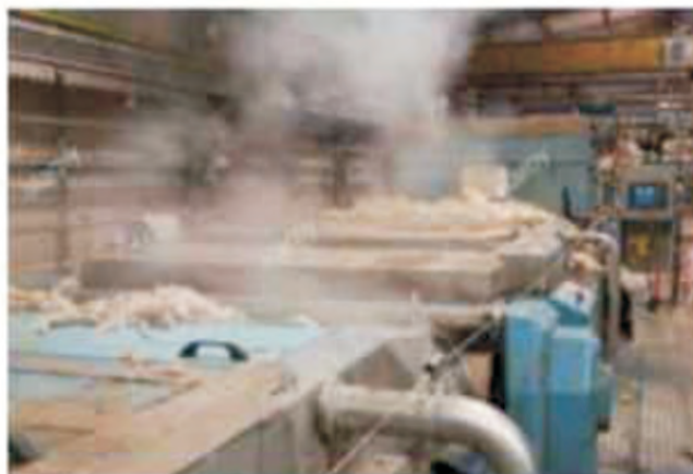
Fig 3.8 (b) Scouring by machines
