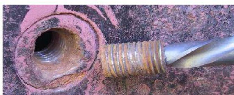
Fig-27 Broken thread
