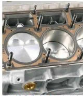
Fig-16 Cylinder head studs
