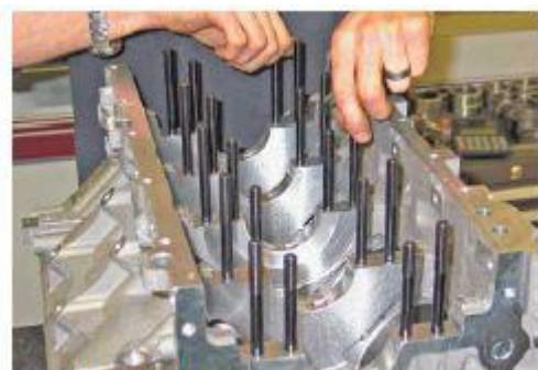
Fig-15 Main studs in engine block
